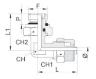
Raccordo a T girevole maschio conico Swivel tee male adapter (taper) centre leg
